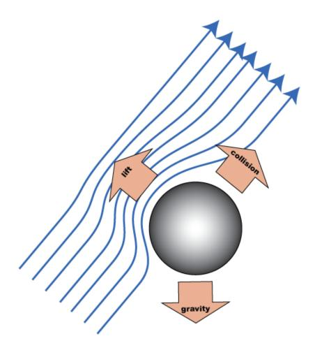
A stream of air travels at an angle up and over a beach ball. The force from collisions with air molecules tries to push the ball in the direction of the stream. The Bernoulli lift force tries to pull the ball directly into the stream. Gravity tries to pull the ball downward. When these three forces exactly cancel, the ball will stay put.
