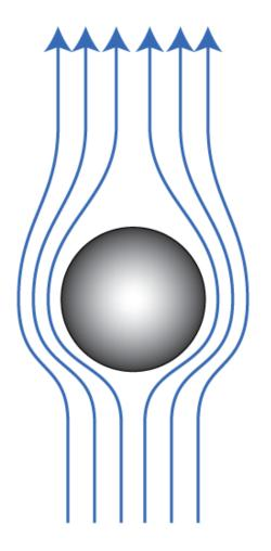
A ball floats in the center of a stream of air. The air hitting it from below cancels the downward force of gravity.
