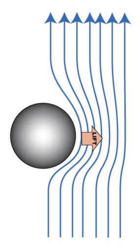
The ball moves to the left of the stream of air. A Bernoulli lift force pulls it back to the center of the stream.
