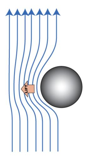
The ball moves to the right of the stream of air. The Bernoulli lift force reverses and the ball is once again pulled back to the center of the stream.
